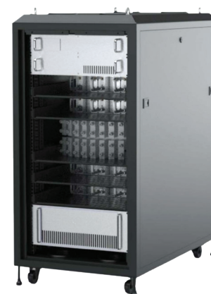
Prototype of a Custom High Power 2.7- 3.1 GHz, 18 kW pulsed radar amplifier system delivered in 20 weeks per customer specifications
